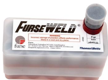
FurseWELD powder shots are selected to match the applicable mould. They are supplied in a box of 10 or 20 units and include the fuse disc to separate the powder from the joint, until the fusion of the powder is activated.
